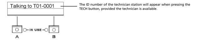
The connection will be interrupted when the TECH button is released.
